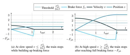
Fig. 4: Brake force and stopping distance
