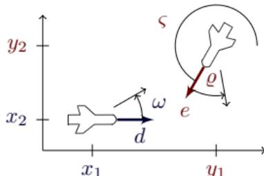
$$\begin{bmatrix} x'_1 = -v_1 + v_2 \cos \vartheta + \omega x_2 \\ x'_2 = v_2 \sin \vartheta - \omega x_1 \\ \vartheta' = \varrho - \omega \end{bmatrix}$$
