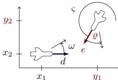
$$\begin{bmatrix} x'_1 = -v_1 + v_2 \cos \vartheta + \omega x_1 \\ x'_2 = v_2 \sin \vartheta - \omega x_1 \\ \vartheta' = \varrho - \omega \end{bmatrix}$$
