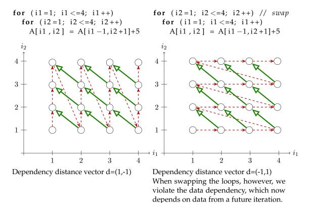
Note that the loop iteration order in the right example would useful for caches, because the consecutive items in cache lines are accessed subsequently, so there is a good cache hit rate. In the example on the left, elements in the cache line are accessed only very late, i.e., after walking all values of i2. For large matrices (here it's just 4) this means that the data will have been cleared from the cache again before accessing the second element in the cache line.
