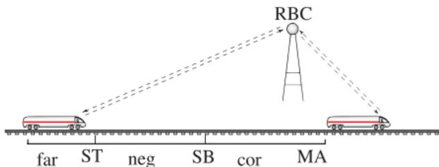
$$\underbrace{[\text{if}(z > SB) a := -b; z'' = a]}_{\text{hybrid program}} v^2 \leq 2b$$
