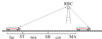
$$\frac{v \geq 0, z < MA \vdash t \geq 0 \quad \frac{v \geq 0, z < MA \vdash -\frac{b}{2}t^2 + vt + z > MA}{v \geq 0, z < MA \vdash \langle z := -\frac{b}{2}t^2 + vt + z \rangle z > MA}}{v \geq 0, z < MA \vdash t \geq 0 \wedge \langle z := -\frac{b}{2}t^2 + vt + z \rangle z > MA}$$
