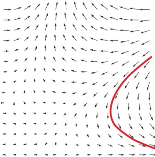
$$\begin{bmatrix} y'(t) = f(t, y) \\ y(t_0) = y_0 \end{bmatrix}$$
