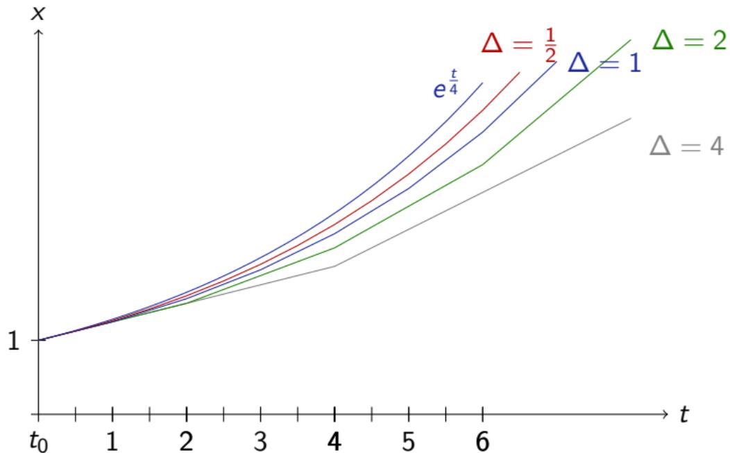
$$\left[ \begin{array}{l} x'(t) = \frac{1}{4}x(t) \\ x(t_0) = 1 \end{array} \right] \rightsquigarrow \left[ \begin{array}{l} x(t + \Delta) := x(t) + \frac{1}{4}x(t)\Delta \\ x(t_0) := 1 \end{array} \right]$$
