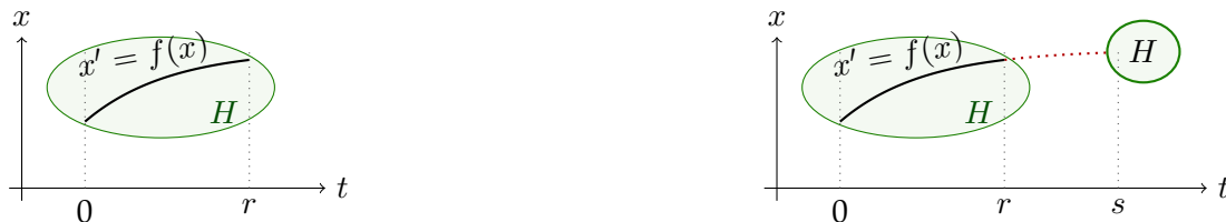
Figure 2: System x' = f(x) \& H follows the differential equation x' = f(x) but cannot leave the (shaded) evolution domain H .
