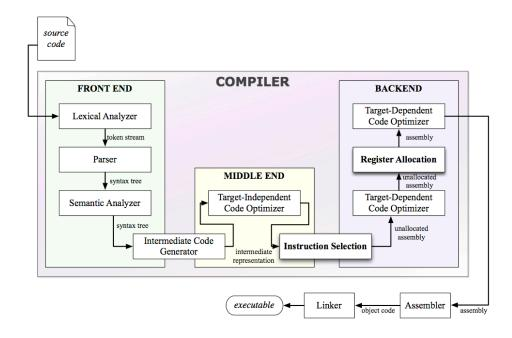
Figure 1: Structure of a typical compiler<sup>1</sup>
